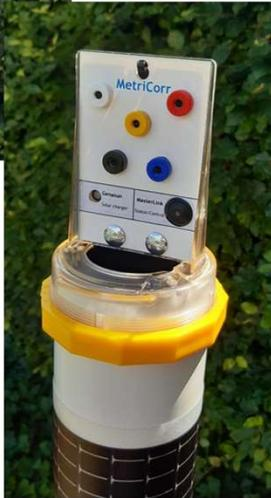
Thickness Corrosion rate: ER probe
